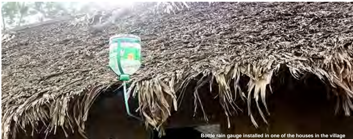
Bottle rain gauge installed in one of the houses in the village
